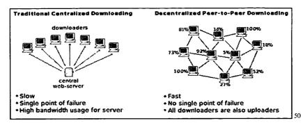
The illustration above shows how P2P sharing is different and more effective than the traditional centralized downloading system. The piecemeal sharing used in P2P networks allows a user to download pieces of a file from many other users, rather than all at once from one central location. File sharing is faster because each downloader is also an uploader, meaning users can share pieces of downloaded files without waiting until they obtain the entire file.
